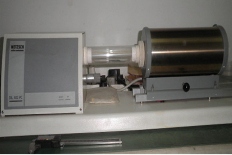
Fig. 2.3 DL402PC thermal conductivity measurement equipment
