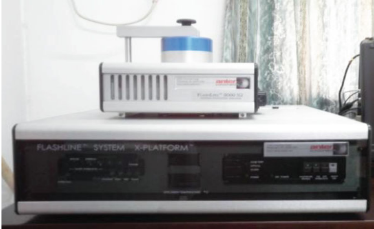
Fig. 2.2 Flash method equipment for measuring thermal conductivity
