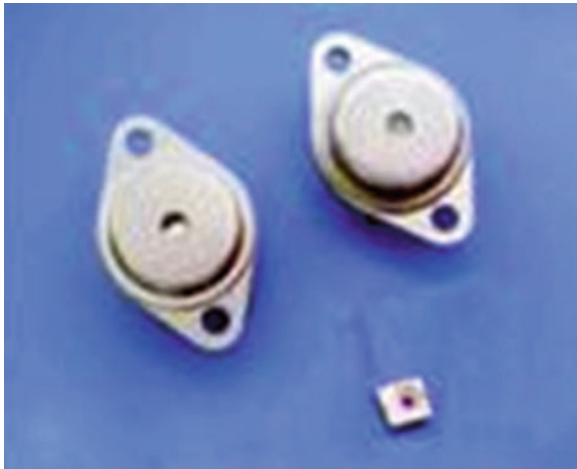
Fig. 1.3 TO header tube socket made of copper material
