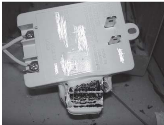
Figure 10.4 Effect of overload current in a transformer that is only short-circuit protected.
