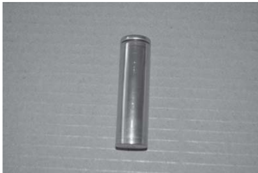
Figure 9.2 A cylindrical lithium-ion cell.
