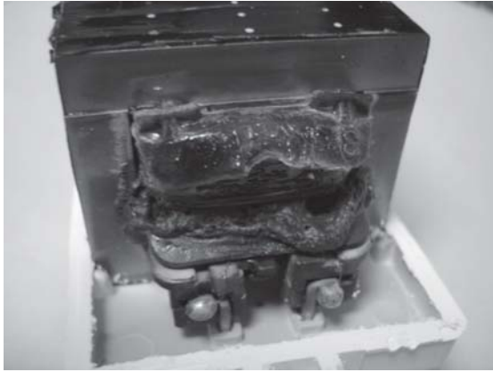
Figure 10.5 Effect of the overload current in a transformer with a thermal cutoff that is incorrectly rated.
